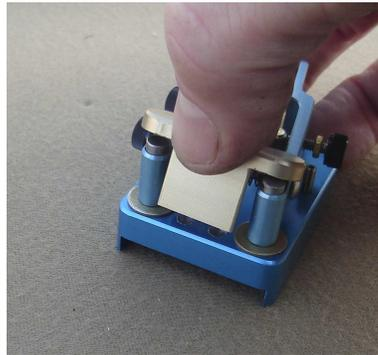
Turn the paddle over & thread the 6-32 x 1/2 pan screws thru the holes in the base into the pin retainer. Note that one hole has a spot face in the anodize; this is for ground connection. Tighten both screws.
