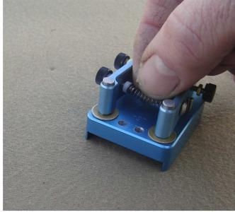
Next fit the pin retainer over the dowel pins; make sure you have the retainer **perpendicular** to the base & press it over the pins with your fingers - snug fit.
