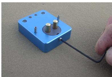
Turn the base over and loosen the 4-40 screws holding the terminal lugs, and spread the lugs apart & retighten. The posts may bind and tighten, or you may need to hold them. Turn the base on edge & hold the post with needle nose pliers while tightening the screws with a Philips screwdriver. You can put tape on the jaws to protect the brass, or simply use care.
