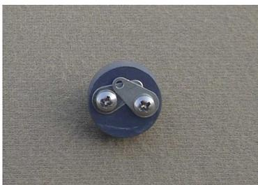
Start the insulator assembly into the bore in the base, with the notch aligned towards the edge of the base and the set screw hole.
