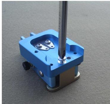
Turn the paddle over & adjust the spring force & contact gaps to your taste & lock with the 3/16 nuts & supplied wrench.
