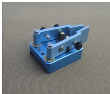
The spring sits tucked in between the levers close to the pin retainer; now is the time to install it while there is room for your fingers. Slide one end over the 7/16 pan screw in the left lever & the other end over the adjuster screw up against the Delrin washer.
